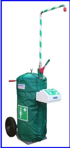
**GENERAL:** the STD 40 K (pictured right) is an unheated safety shower and eye-wash station intended for temporary use, capable of delivering a deluge of water for up to 1 ½ minutes. This unit is easily filled by connecting to a mains water supply via a 15 mm hose; it is then simply wheeled to its required position.
